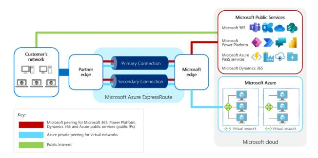
ExpressRoute doesn't encrypt or filter traffic natively (unless you use <a href="ExpressRoute Direct with MACsec">ExpressRoute Direct with MACsec</a> <a href="Enabled">enabled</a>). It only establishes a private connection between the Microsoft and customer datacenters through their connectivity provider.
